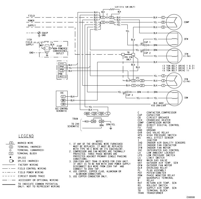
Fig. 83 - 48TC Typical Unit Wiring Diagram - Power (A06, 208/230-3-60)
